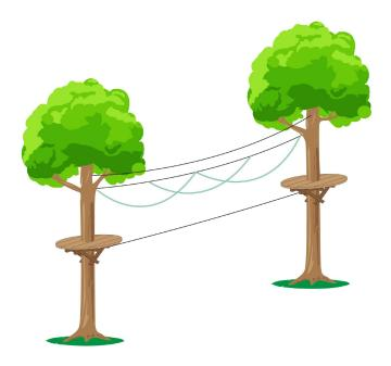
The Droopy Three-Line challenges participants to figure out how to keep tension on the ropes hanging down, in order to stay balanced as they traverse across the foot cable. The Droopy Three-Line provides a moderate level of difficulty.
