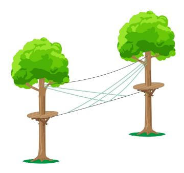
This variation of the standard Pirate's Crossing provides an additional hand line, yet is still quite challenging! It starts off easy but becomes very unstable and shaky when you reach the crux (the center.) The hand-lines are typically adjustable and can be loosened or tightened to change the level of difficulty.
