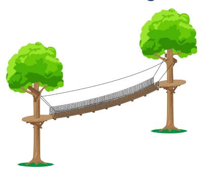
The Catskills Bridge is an Appalachian Bridge with cargo nets in place of the support ropes. The cargo nets add great aesthetics to the bridge. There is enough security inherent to this design that this bridge can be used off of the course for pedestrian creek crossings.
