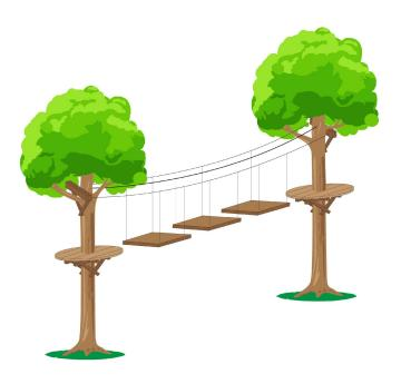
The Floating Islands are a dynamic challenge! These large platforms really swing! The crux is timing the jump from platform to platform just right. Three platforms is the standard for this station, but two or four is also possible. Three platforms put the spacing at about 25' between trees. This is one of the harder elements listed in this guide.
