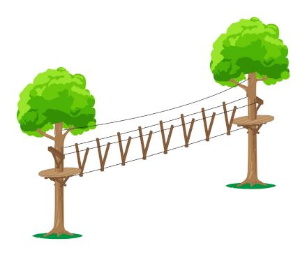
The Timber Burma uses timbers in place of the support ropes on the classic Burma Bridge element. The timbers provide much more stability than the ropes, making this bridge great for any length span. Aside from the Sky Bridges, this is the easiest bridge in the guide.
