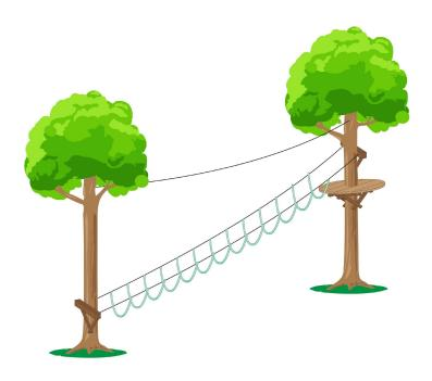
Inclining Burma Loops provides a visually appealing, alternative approach to accessing the course. Instead of using a ladder, the loops start at ground level and participants elevation as they climb the element. This element is challenging.
