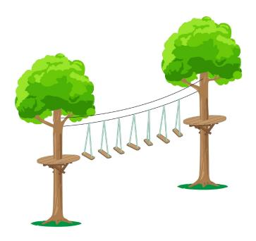
The Bosun's Chairs is an old favorite from our High Challenge Selection Guide. The Bosun's Chairs element is a difficult traverse for more challenging courses. We recommend it for spans less than 25'. A good deal of upper body strength is required despite the foot plank. It is one of the most difficult stations listed in the guide.
