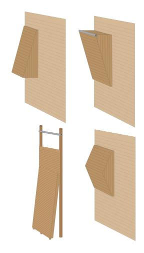
These climbing features can be added to a flat wall to modify the climbing challenge. The inclining panel makes the wall significantly easier, and the overhangs can make the climbing very difficult! These features are available in a wide variety of sizes, and can be added to existing towers to spice up an older design. Four-sided towers can have seamless inclines and overhangs installed (see page 6).
